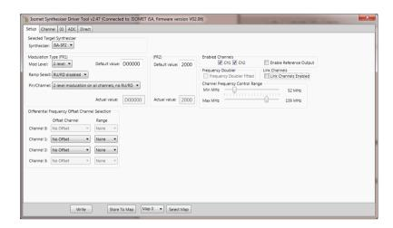
For basic single tone (static frequency) operation, use the default values for the **Modulation Type** (FR1) and (FR2) panels as shown above.
