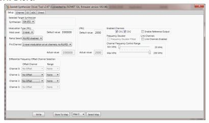
b) The sweep modes are selected under the *Channel* tab.
