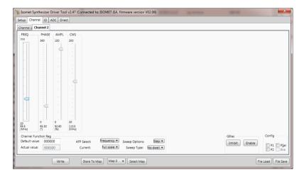
Step mode may be applied to the Frequency, Amplitude or Phase. In the example screen shot above, frequency will switch between 69.5 and 110.5MHz Also *Full scale* amplitude selected. *Dwell / No dwell* has no function.
