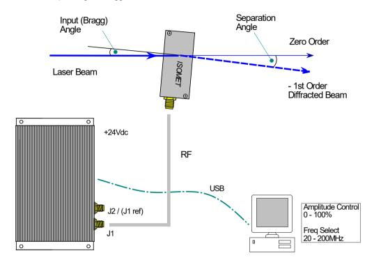
The input Bragg angle relative the optic face normal is:
