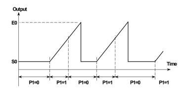
A **Dwell** sweep only returns to the S0 start value after a falling edge transition on the appropriate profile input
