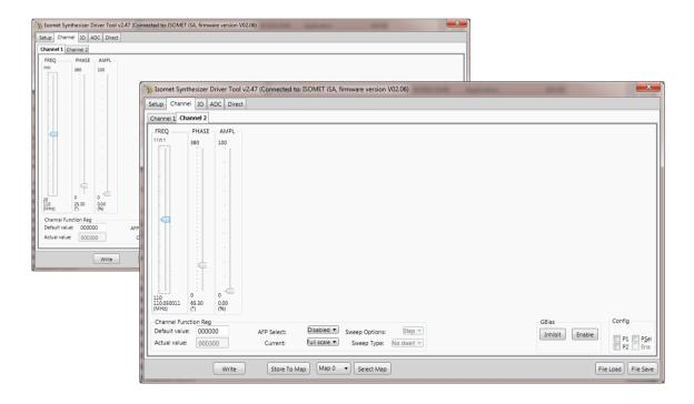
Tip: For precise control, set the Channel Frequency sliders to minimum using the mouse and then use the arrow keys to increment (see table page 6)
