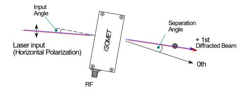
Input the light source and rotate the AOTF so that the incident beam is in the correct orientation and angle. Ensure the light beam is in the centre of the aperture. Start with the input beam at normal incidence. A slight rotation such that the beam is directed away from connector end of the AOTF will avoid back reflection into the source
