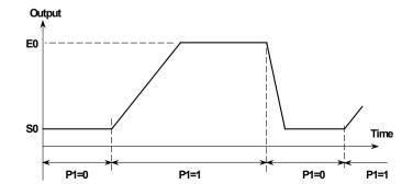
(Both plots show a Ch1 ramp, controlled using input P1)
