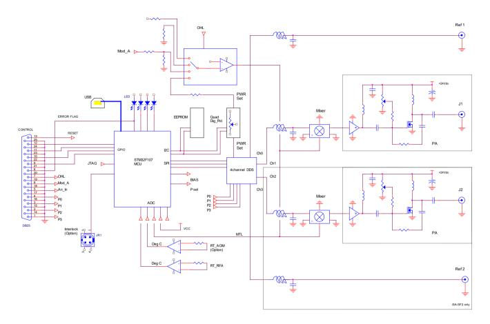
Figure 5: Driver Block Diagram
