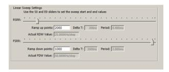
The RSRR slider defines the duration of the rising slope increment.
